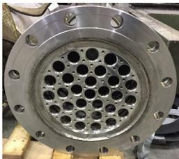
Multiple membranes mounted inside a common housing to minimize footprint
